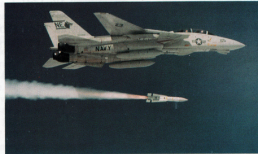
An F-14A from the Wolfpack of VF-1 launching a Phoenix missile during 1989 workups
