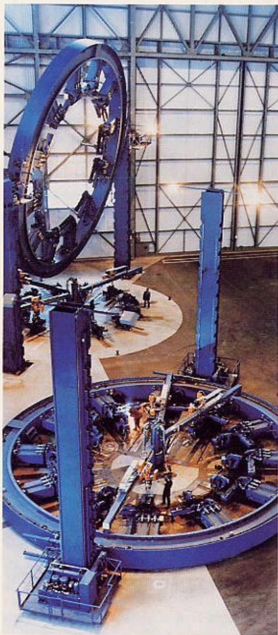
Automated submarine frame making machine at Quonset Point, R.I.
