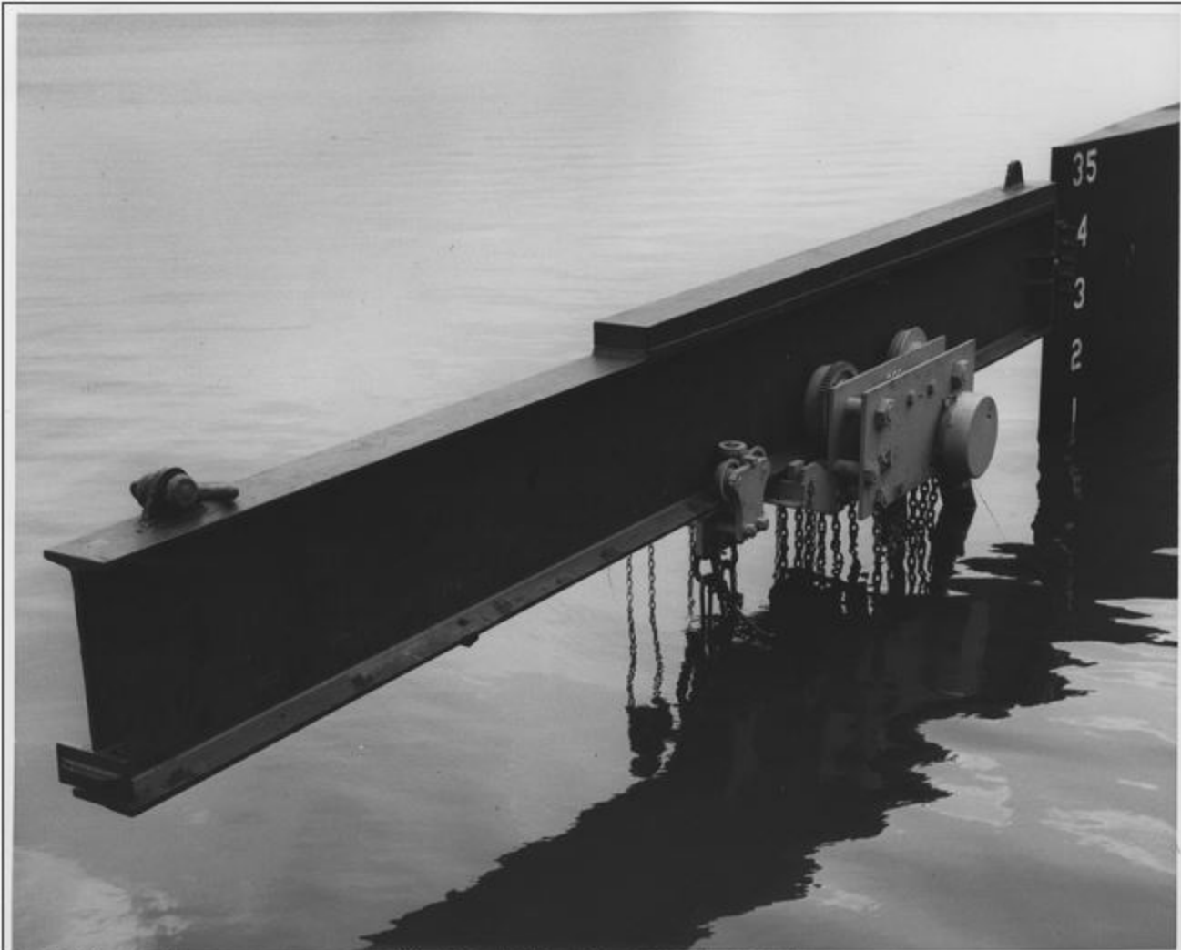
SSBN-600 BRIDGE CRANE ASSY RIGGED FOR PROPELLER REMOVAL
