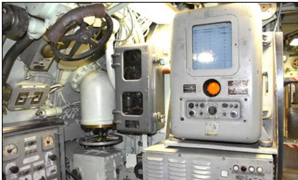
Left to Right: Sounding sonar set on aft wall of chart area. Older style of pen and ink plotter; Starboard side overhead. It wouldn't be a submarine without a profusion of overhead cables.
