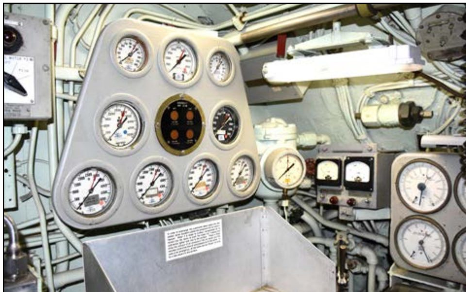
Left to Right: Directly behind the pilots are the high pressure air bank gauges. HP air was used to empty ballast tanks. This late installation allowed push button control of the HP air manifold; On the starboard side of the control room is the chart area and sounding gear.
