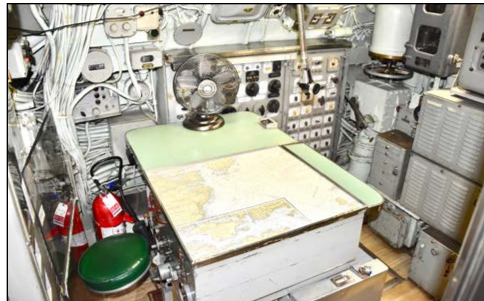
Left to Right: Directly behind the pilots are the high pressure air bank gauges. HP air was used to empty ballast tanks. This late installation allowed push button control of the HP air manifold; On the starboard side of the control room is the chart area and sounding gear.
