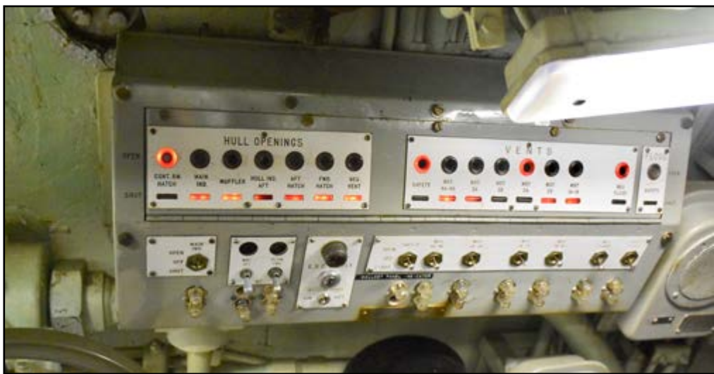
Left to Right: Just to the left and overhead of the pilot station are the all important hull openings and vents panel. Even at this point, the WWII red and green lights have been replaced by circle and bar symbols with all red lights. During WWII, red night vision goggles made it difficult to see the green lights; On the port side hull next to the pilot station are the trim tank indicators.
