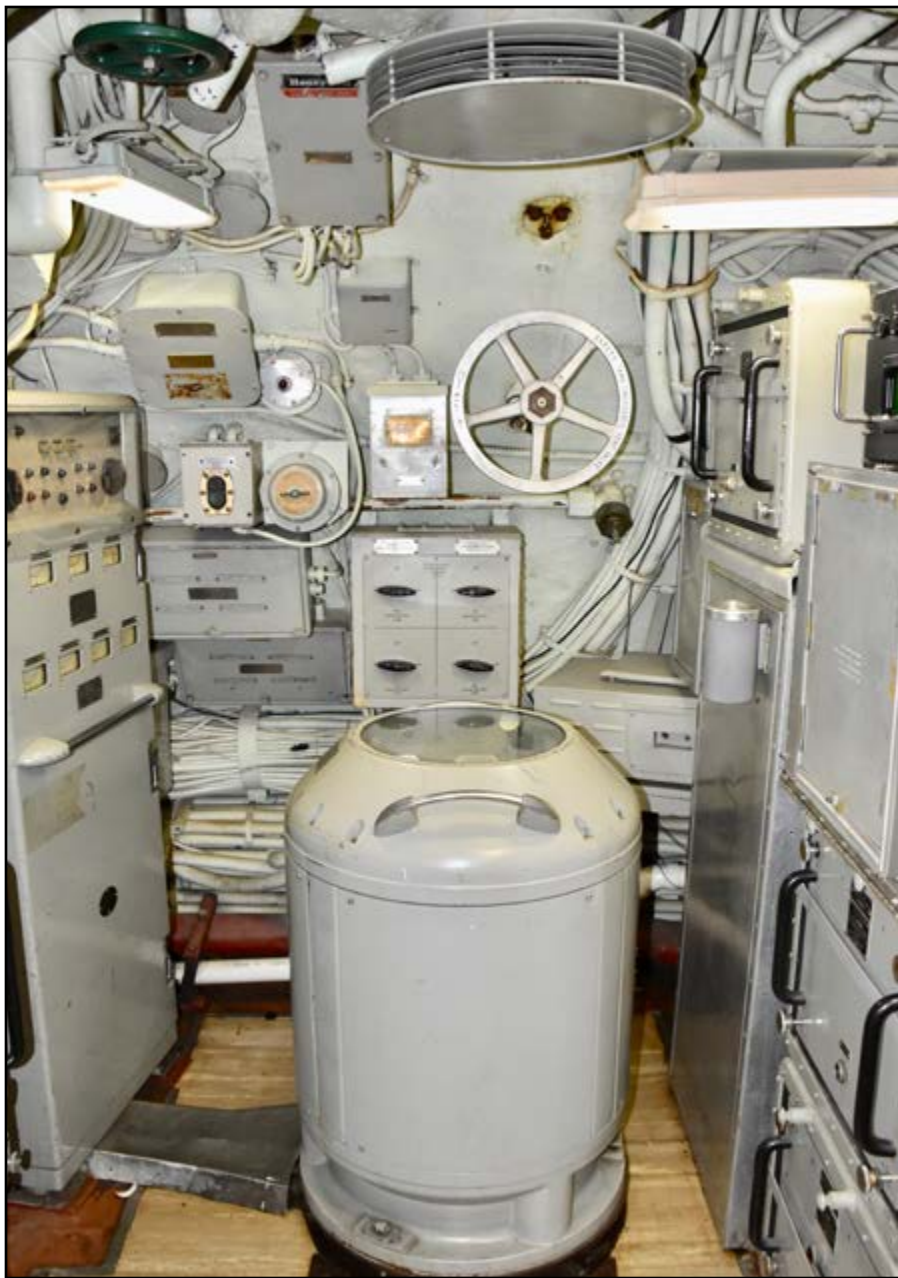
Opposite the sonar room, the ship's Sperry gyrocompass and associated electronics are installed.
