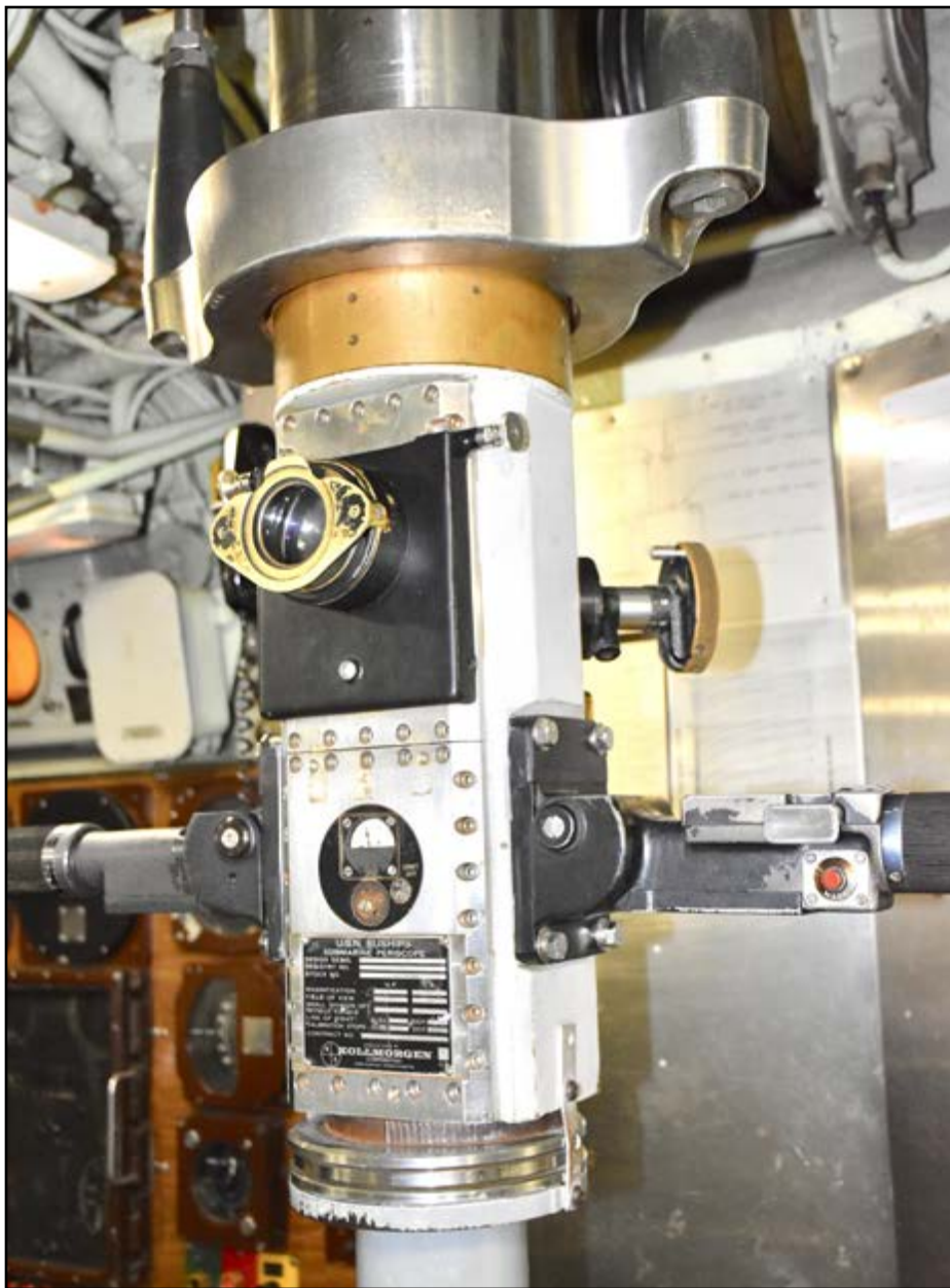
Control room center is where the single periscope is housed (central round circle in Cont Rm).
