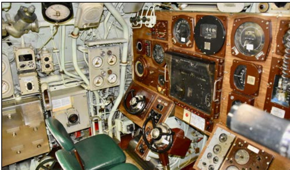
Left to Right: View of Albacore's unique "pilot" station. The seat is facing forward. The closest control wheel can be employed for single pilot mode. Alternatively, the load can be split between two pilots using the secondary control wheel. The large black gauge, reading 000 is the digital depth gauge. Other instruments indicate heading, speed and angles (Cont Rm on the diagram); Another view of the piloting station. The starboard wheel moves forward and backward when in single pilot control mode. The larger black panel between the two wheels is the mode selection switch. These are the much improved Ph. 4 instrument suite.
