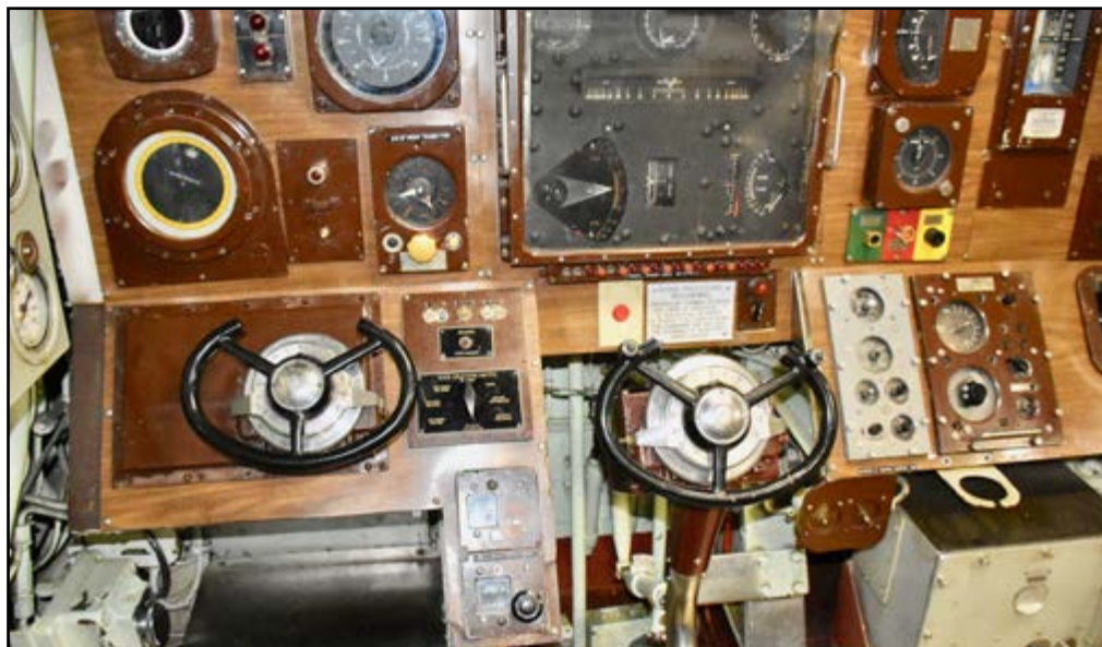
Left to Right: View of Albacore's unique "pilot" station. The seat is facing forward. The closest control wheel can be employed for single pilot mode. Alternatively, the load can be split between two pilots using the secondary control wheel. The large black gauge, reading 000 is the digital depth gauge. Other instruments indicate heading, speed and angles (Cont Rm on the diagram); Another view of the piloting station. The starboard wheel moves forward and backward when in single pilot control mode. The larger black panel between the two wheels is the mode selection switch. These are the much improved Ph. 4 instrument suite.
