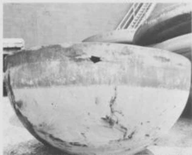
AS-FORMED HEAD (ARROW INDICATES SURFACE CRACK)
