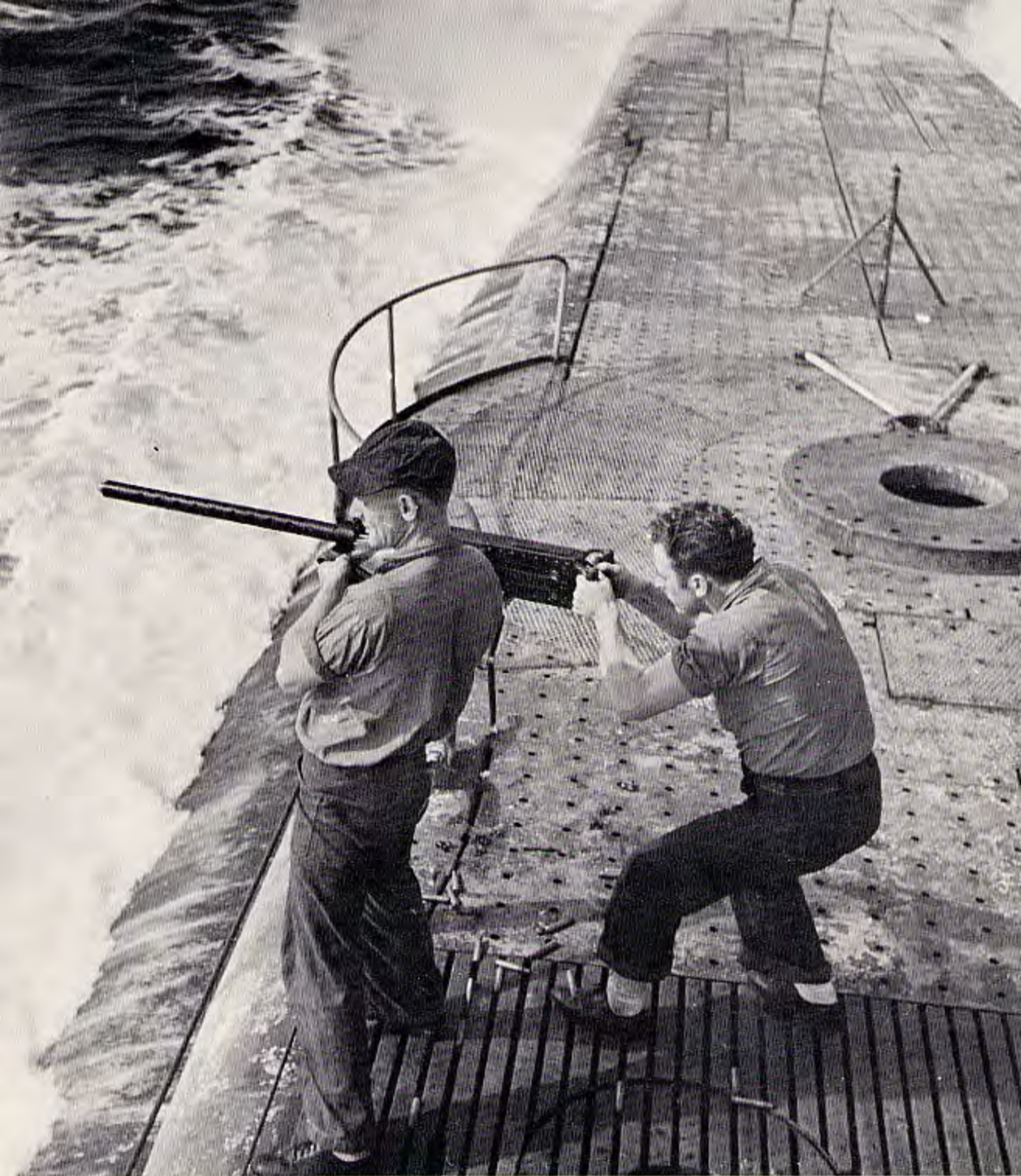
Batfish crewmen fire .50 caliber machine gun at floating mine Japanese had let loose in South China Sea. For surface battle, Batfish mounted a 5-inch 25 cal. gun; one 40-mm gun; and two .50 cal. machine guns.
