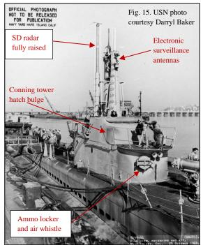
the boat's air whistle. *Balao* has also been refitted with a new number one periscope which in addition to the optics had a small range only radar transmitter/receiver built into the head. This ST radar eliminated the guess work involved in getting an accurate range to a target while making a submerged approach. It was a modification that was highly coveted by the boat commanding officers, but its initial availability was somewhat limited.
