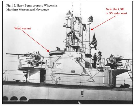
distinguishes these boats as the Type 3. Carbonero (SS-337) was the first boat with a Type 3 and all subsequent EB boats were built this way. Manitowoc made the shift to the Type 3 with Macabi (SS-375) in May 1944. Figure 12 is a September 1945 shot of *Mero* and is a very good representation of a Type 3 boat. The LF loop has been moved aft between the shears and the radar mast (in this case the brand new SV) and she sports two 40 mm gun mounts. A late war
