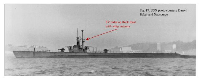
Her wartime SD radar has been replaced with the new and much more capable SV with its large screen dish. The SJ mast has been moved aft of the shears, and a whip style radio antenna has been
