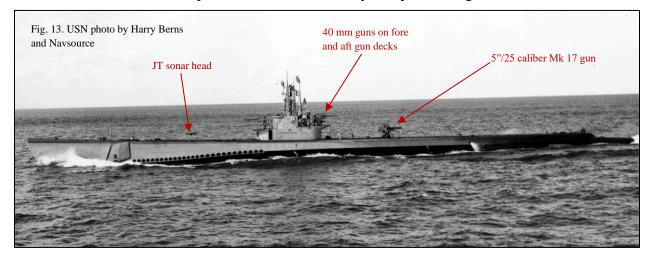
Type 3 configured *Macabi* (SS-375) on trial runs in Lake Michigan in 1944. The T-shaped bar on her forward deck is the rotating head for the JT sonar, a passive listening array meant to supplement the standard QB/QC transducers mounted on retractable posts underneath the forward torpedo room on the keel.
