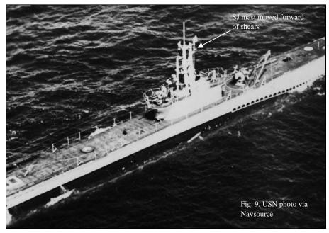
mast aft of the shears and out of the way on the bridge. However, starting with Bugara (SS-331) all subsequent EB boats were built with the SJ forward (the sited sequence may have started with Brill (SS-330), but her as-built configuration is not yet clear). Manitowoc made the switch to SJ forward starting with Lizardfish (SS-373) in March 1944. This arrangement of the SJ forward, followed by the two scopes, then the
