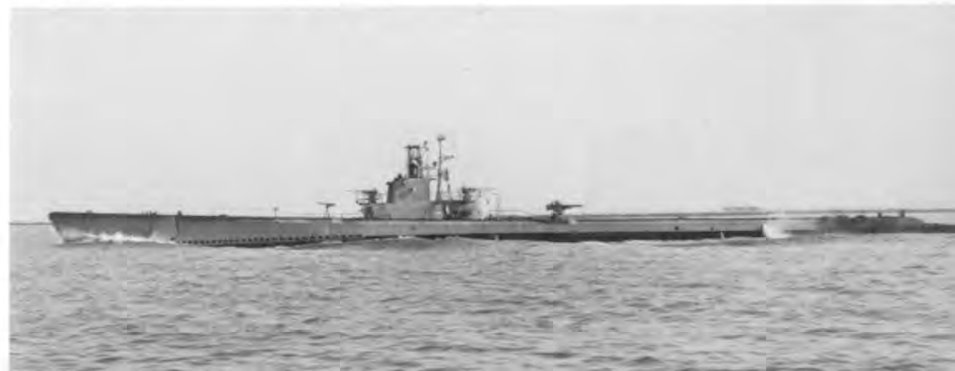
(Above) This view of USS Wahoo (SS238) taken 14 July 1943 shows the first major bridge alteration given to the early fleet-type submarines. A heavier 4"/50 deck gun has been mounted forward and a 20mm has been mounted on the forward and aft bridge platforms (barrels are removed). (Below) Most fleet-type boats finished the war outfitted similar to this 20 July 1945 shot of USS Mingo (SS261), mounting a 5"/25 aft, 40mm on the bridge platforms and in many boats a 20mm was placed over the main gun foundation forward.
