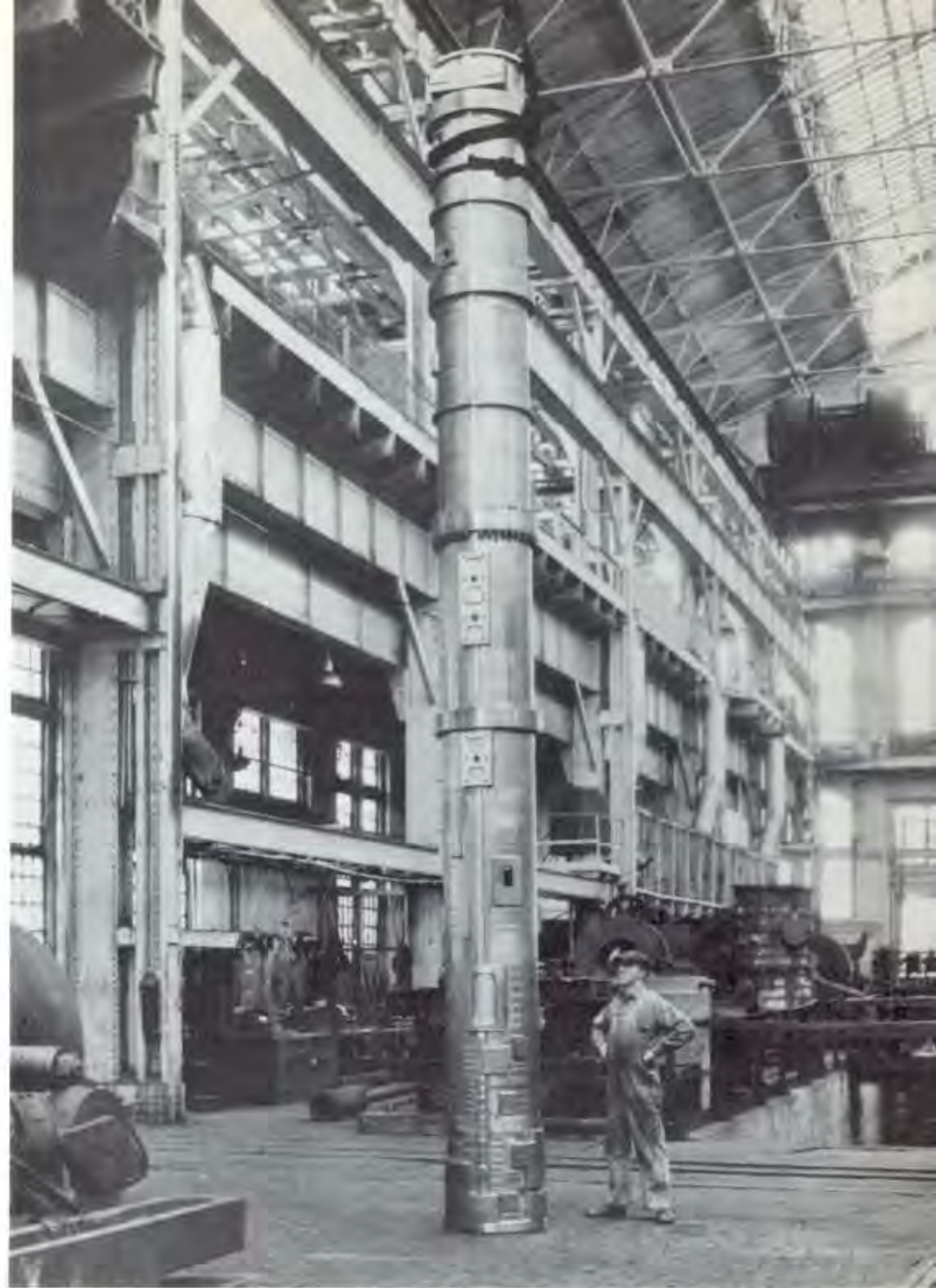
(Left) Perspective view of a 21" submerged torpedo tube (MK32-39). (Above) This corrosion-resisting steel torpedo tube was fabricated by the Midvale Steel Co. The massive size of a submarine torpedo tube is evident from the workman standing alongside.
