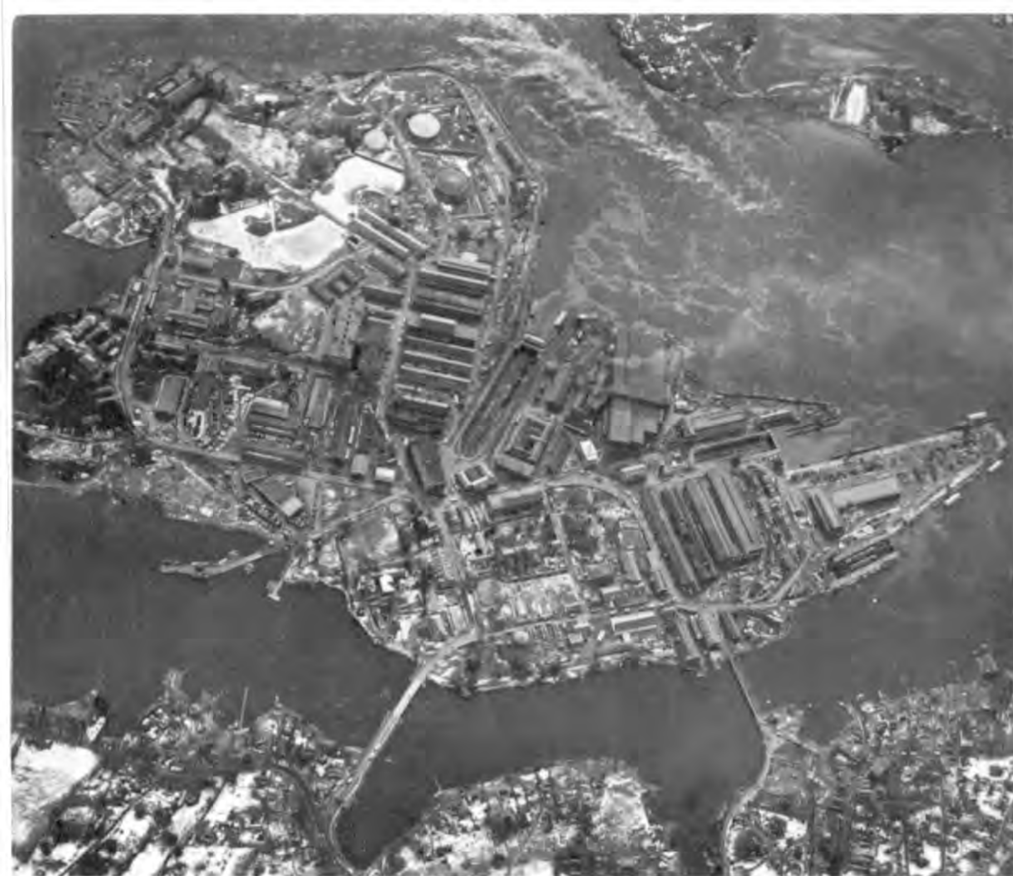
The Navy Yard at Portsmouth, New Hampshire where Bowfin was built. The yard, on an island in the Piscataqua River, is just off Kittery, Maine. The shipways, which are covered, are just to the right of the graving dock in the center of the island.
