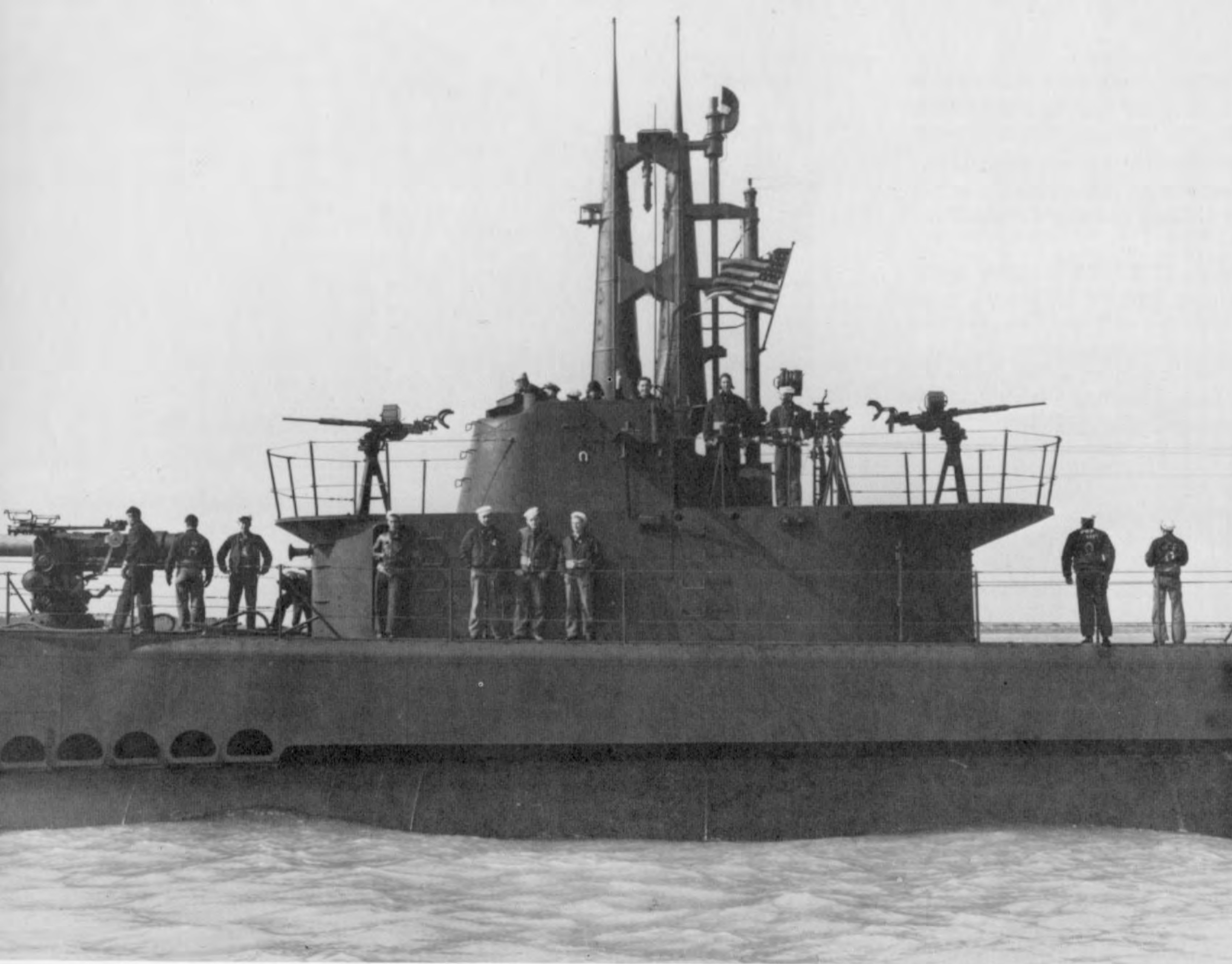
Close-up of USS Hardhead (SS365) showing port side of bridge in April 1944 configuration.
