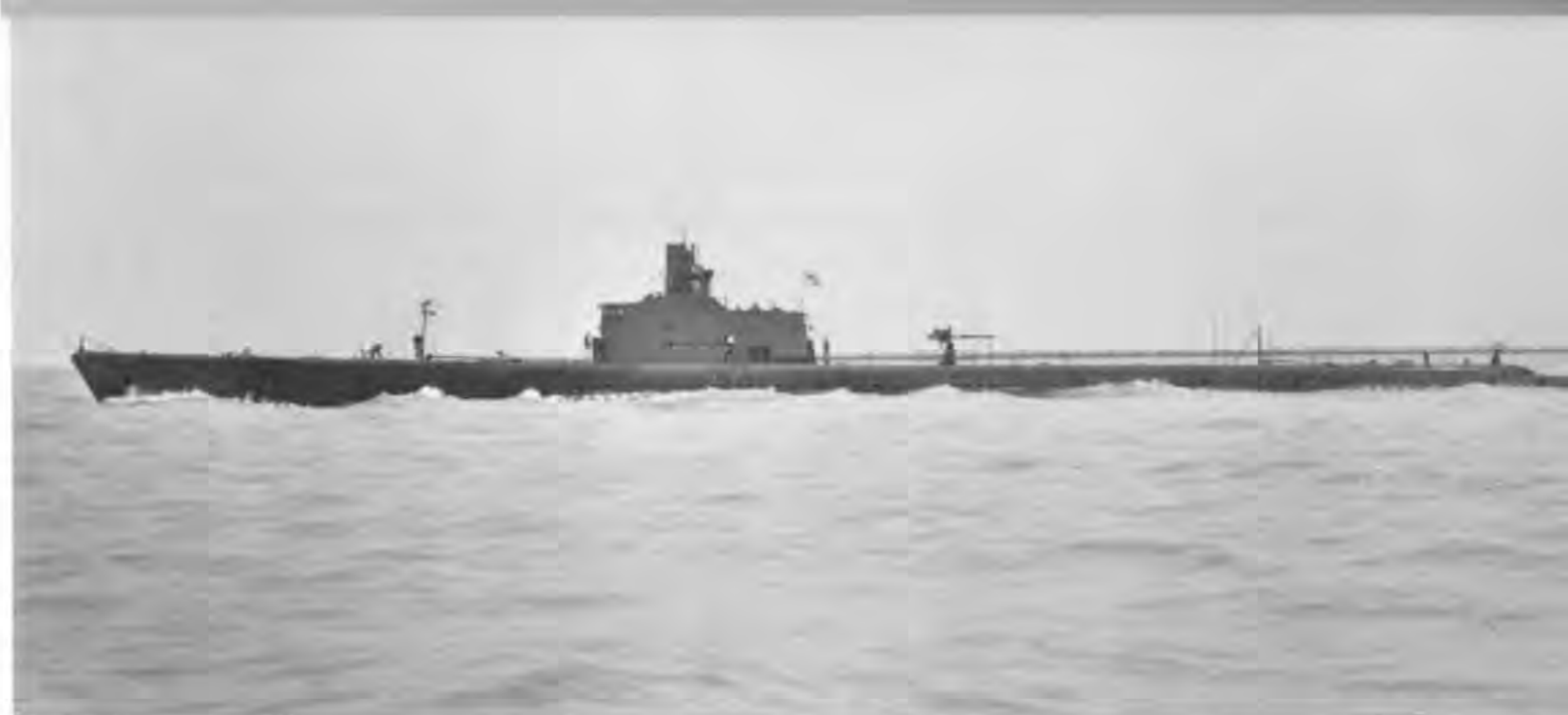
Original bridge design for early fleet-type boats is shown in this 6 April 1942 view of USS Trigger (SS237). Original 3"/50 deck gun proved too light for surface targets.
