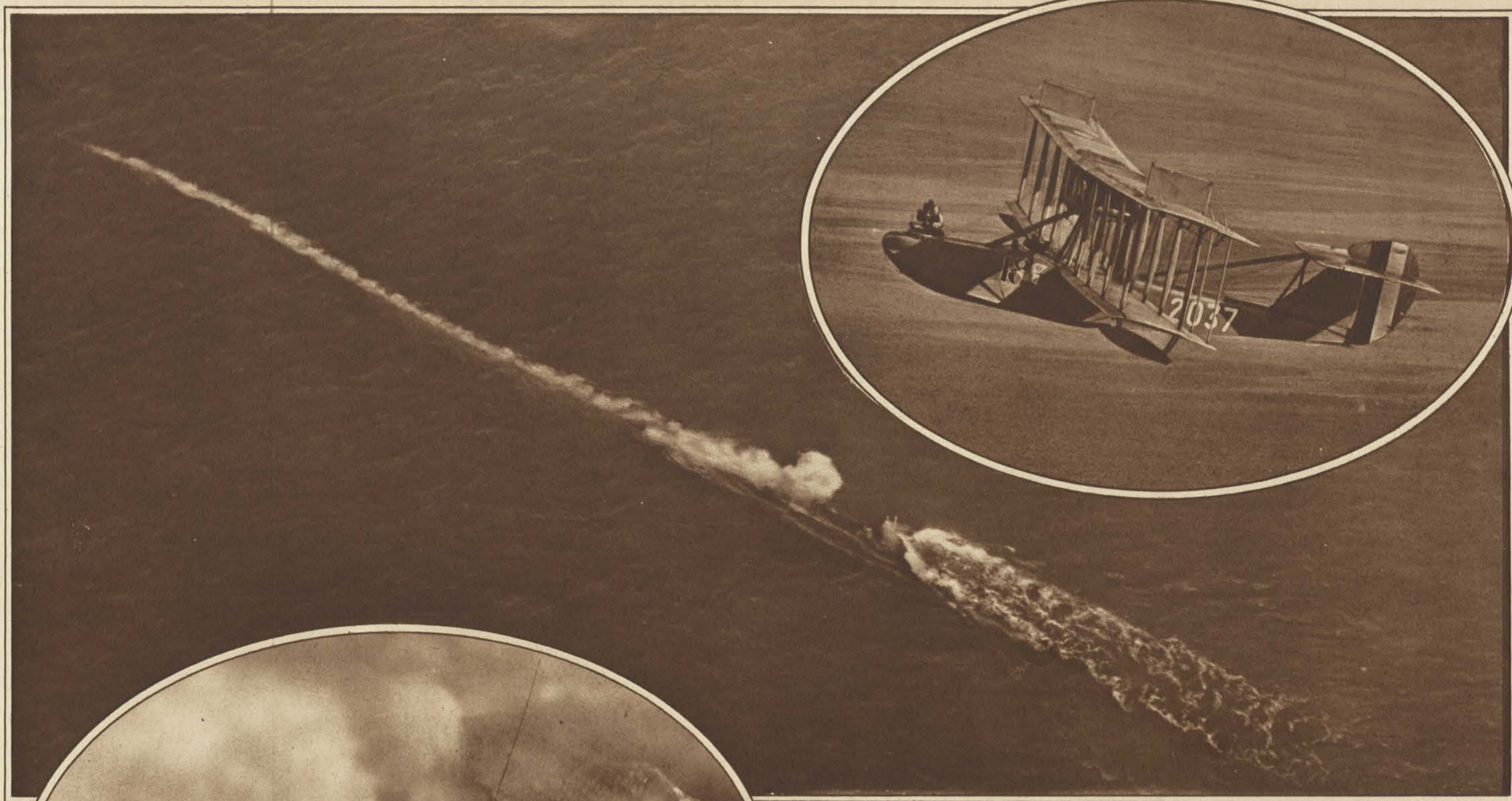
A SUBMERGED AMERICAN SUBMARINE FIRING A TORPEDO, AS SEEN FROM A UNITED STATES NAVAL SEAPLANE AT AN ELEVATION OF NEARLY 1,000 FEET. The Compressed Air from the Torpedo Tube Has Just Risen to the Surface Where It Has the Appearance of a Cloud of Steam. The Wake of the U-Boat's Periscope Also Appears Plainly.
