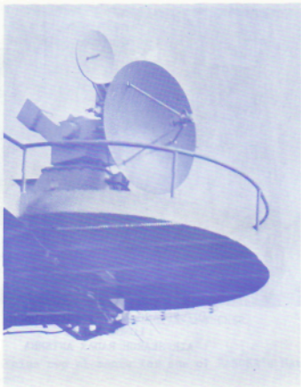
AN/SPN-42A AIRCRAFT LANDING SYSTEMS ANTENNAE (CLS)
