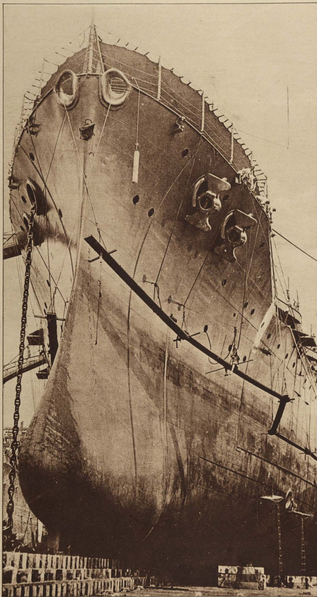
THIS TOWERING HULL OF THE DREADNOUGHT OKLAHOMA HAS A KEEL THAT IS VERY HEAVILY WEIGHTED TO OFFSET THE PONDEROUS ARMAMENT ABOVE.
