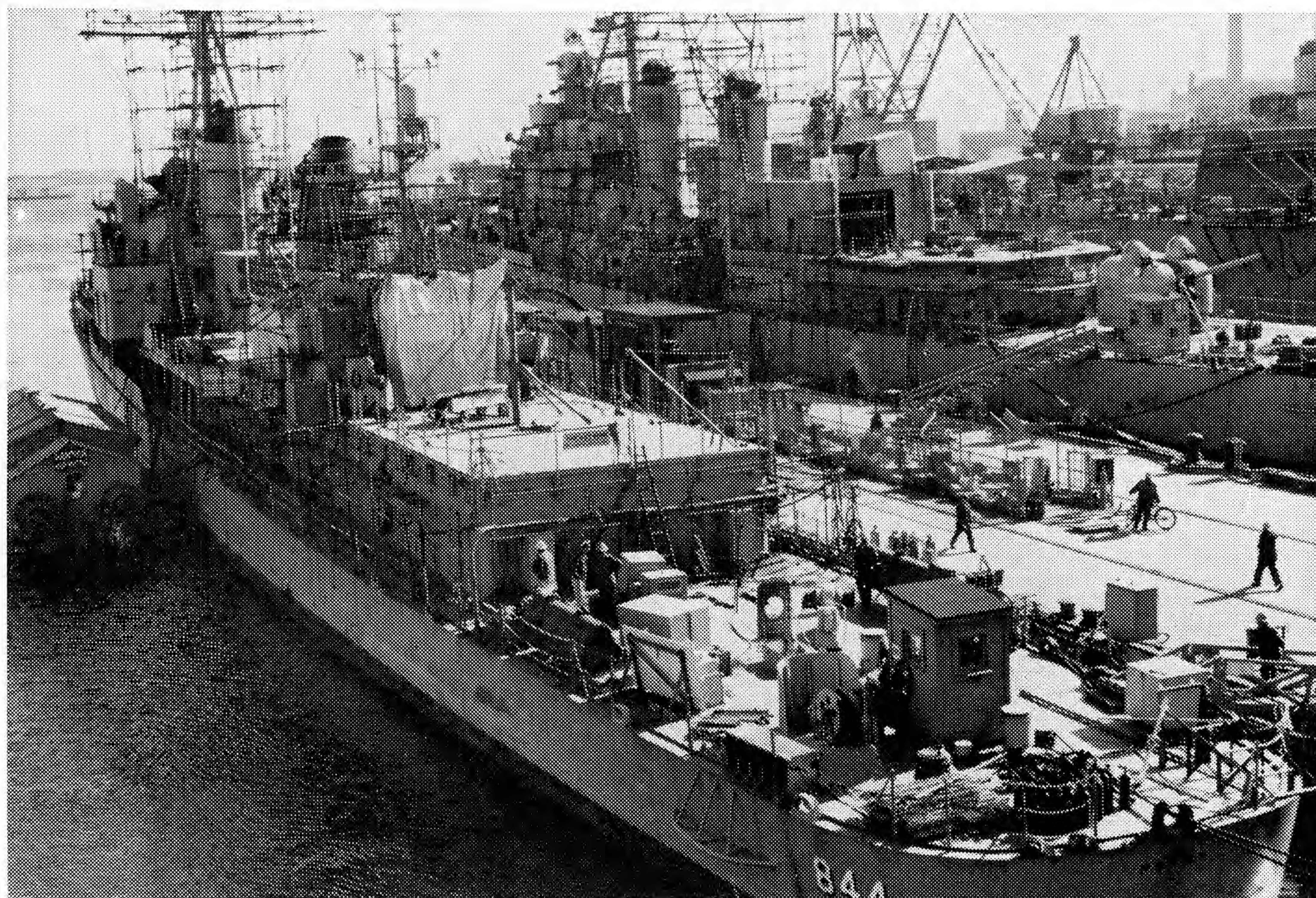
Not only have guns given way to missiles but also to other weapon systems. During her FRAM overhaul the USS Perry (DD-844), for example, lost two of her six 5"/38 guns.
